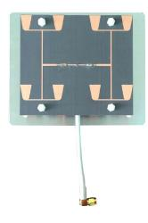
Model: FTD-3742IPB15V30Name: Built-in Antenna
